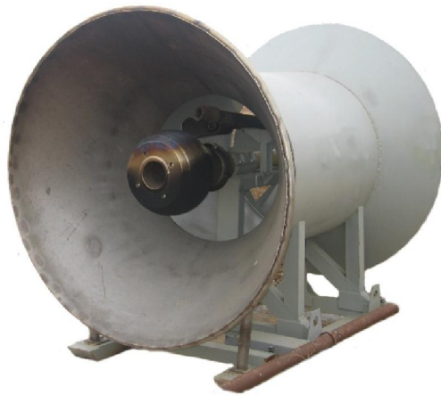
Horizontal burners For the combustion of reservoir mixture and waste gases during the flowline purging of gas well clusters.
