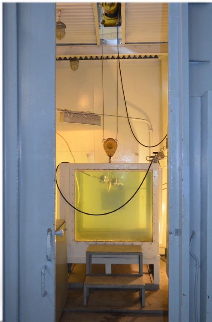
Pneumatic and hydro testing , P_{max} = 105 \text{ MPa}
