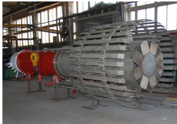
Flares Smokeless burning without additional air supply
